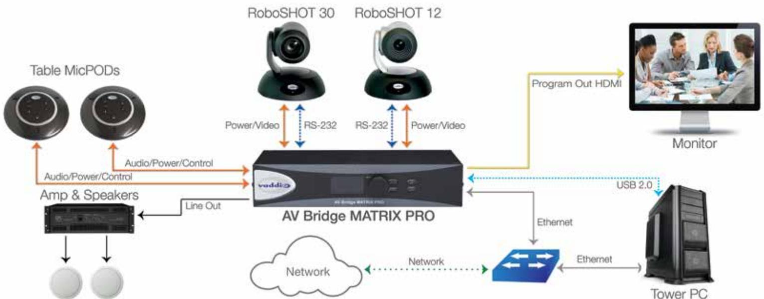
Bridge products offer a flexible AV interface that "bridges" a room's legacy analog audio and video to a PC.
