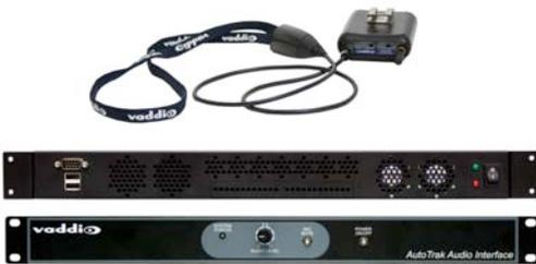
**AutoTrak** combines IR camera tracking and a wireless microphone into one easy to use system designed for the education and distance-learning marketplace. The instructor wears the IR lanyard, with an integrated microphone attached to a belt pack. An IR PTZ camera tracks the IR lanyard, sending commands to the Tracking PTZ camera, keeping the instructor framed in the shot, which becomes the high definition or standard definition video output.
