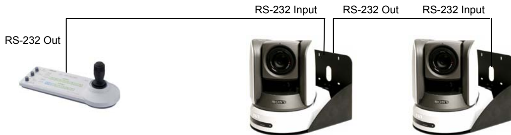
Figure 3: Daisy chain control configuration using two (2) WallVIEW PRO HD1 systems and a single RS-232 output control device. See Appendix 1 for wiring and pin-out information.
