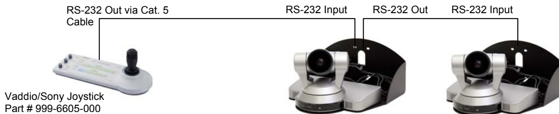
Figure 5: Daisy chain control configuration using two (2) WallVIEW PRO HD1 systems and a single RS-232 output control device. See Appendix 1 for wiring and pin-out information.
