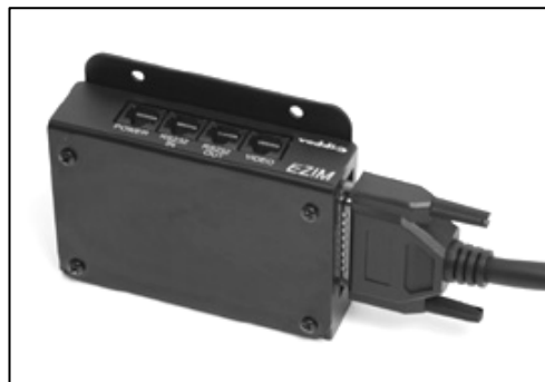
Figure 5: 25-pin connector mounted to EZIM (left) and EZIM mounted to the Wall Mount (right)
