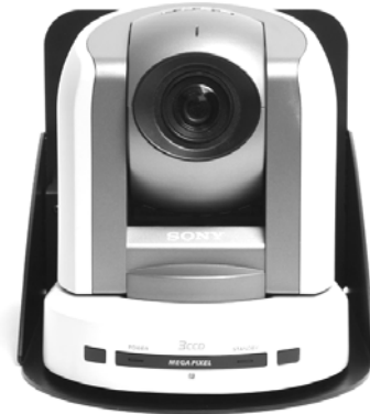
Figure 1: WallVIEW PRO 300 System with Camera, Wall Mount and EZIM (behind camera)
