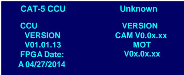
2: If there is an “A” listed before the FPGA date, go back into the Vaddio Loader, choose “Quick-Connect CCU CAT-5(Video ‘A’) in the File drop down menu. If the “A” is not shown on the FPGA date, choose the “Quick-Connect CCU CAT-5(Video) in the File drop down menu.
