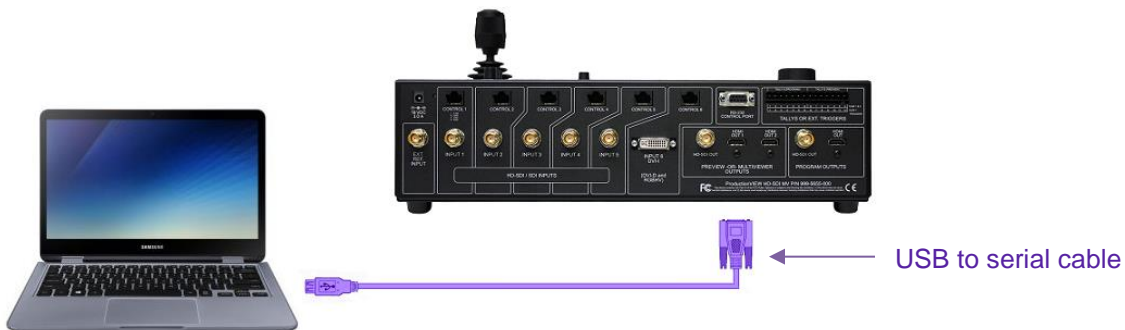
Example connection diagram – your cable color may be less fun.
