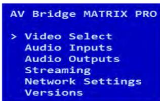
**Video Select:** Control. This menu indicates the current source of the program output with the \* symbol. Use the menu knob and Select button to select a different program source
