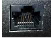
**Damaged** – Some contact fingers are bent and will NOT make reliable contact with the cable connector
