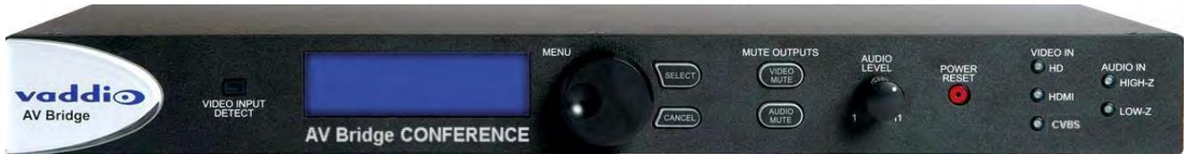
The AV Bridge CONFERENCE offers a flexible A/V interface that is controllable with an embedded web server and the current settings are viewable from the front panel menus. It accepts a multitude of video input resolutions from standard definition composite video (480i/NTSC and 576i/PAL) all the way up to HD 1080p/60 in HDMI and YPbPr, including the most relevant wide-screen and 4:3 VESA type PC resolutions (RGBHV or DVI).
