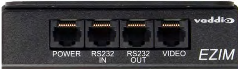
Image: EZIM Top Panel (left to right) and ISO View of EZIM (About the size of a deck of cards)
