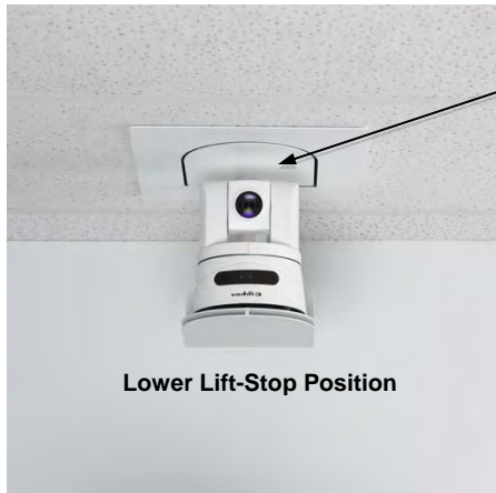
Figure 24: CeilingVIEW HD HideAway Lower Lift-Stop Position Align the upper décor plate to the Trim Ring
