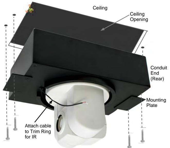
Remove the enclosure and install the spiral wall anchors or any other drywall anchor, like a toggle bolt (not supplied) of the integrator's choice or preference.
