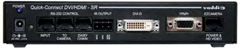
Rear Panel of the Quick-Connect DVI/HDMI - SR Interface (1/2 Rack Width Enclosure)
