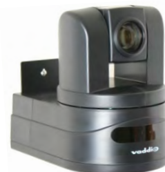
Fig. 6: Completed CONCEAL Wall Mount Camera Bracket Installation
