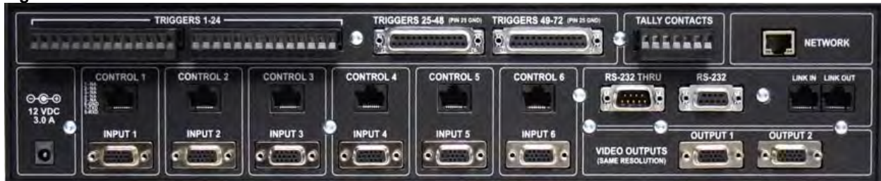
Figure 9: AutoPresenter Back Panel with I/O Information
