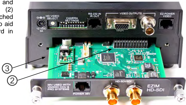
Figure 10: Rear View of HD-18 Showing Insertion of the Slot Card
