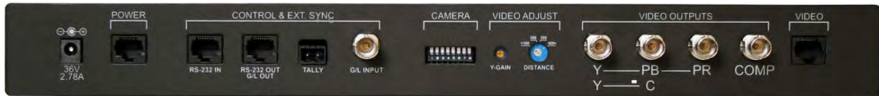
Figure 5: Quick-Connect HD-18 CCU Rear Panel
