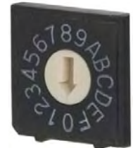
Rotary Switch on Rear of HD-18 Camera
