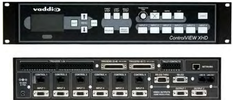
Figure 1: Front and Back views of ControlVIEW XHD.
