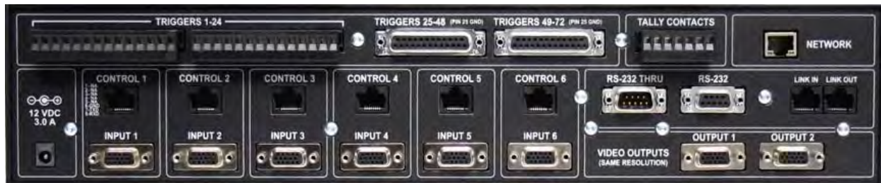
Figure 9: ControlVIEW XHD Back Panel with I/O Information
