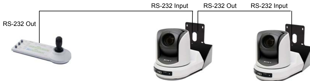
Figure 3: Daisy chain control configuration using two (2) WallVIEW PRO Z330 systems and a single RS-232 output control device. See Appendix 1 for wiring and pin-out information.
