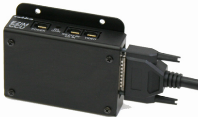
Figure 4: 25-pin connector mounted to EZIM CCU (left) and EZIM CCU mounted to the Wall Mount (right).
