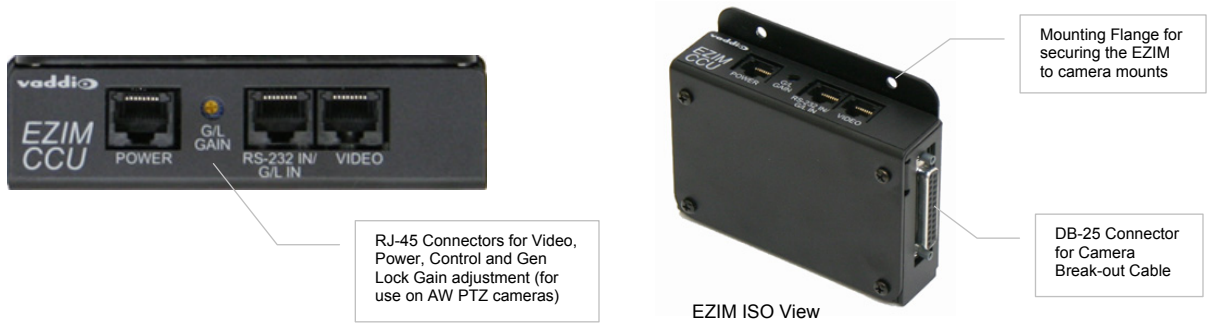
Figure 3: EZCamera Interface Module CCU (EZIM) with three (3) RJ-45 connectors for POWER, RS-232 IN / GEN LOCK and VIDEO (HD or SD), Top View (left) and Isometric View (right).
