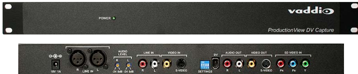
Figure 1: ProductionVIEW DV Capture Front Panel (top) and the Rear Panel Connections (bottom)
