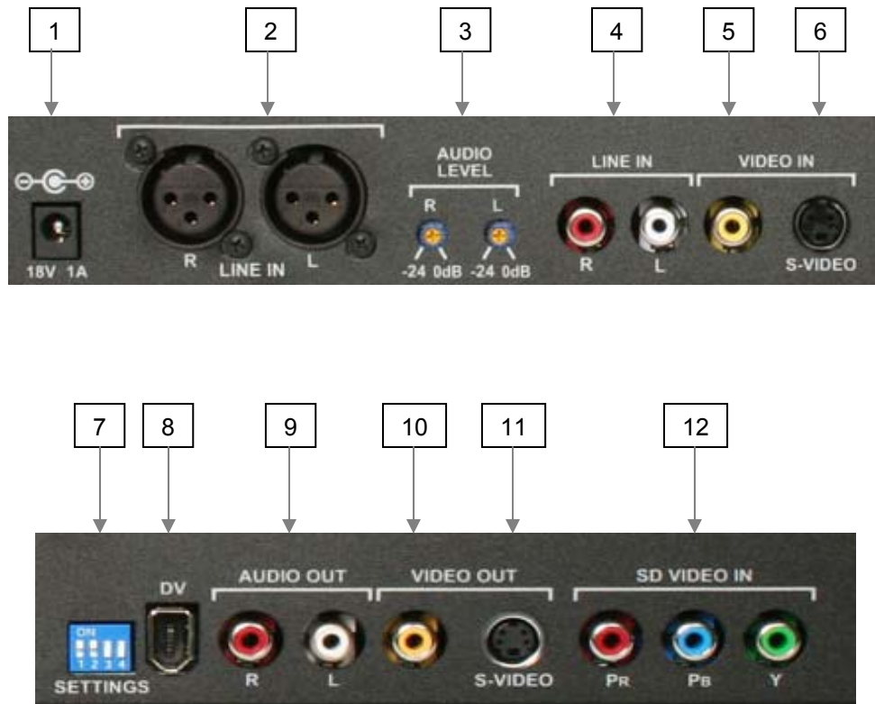
Figure 3: Back Panel Connections Power, audio and video inputs (top), DV, audio out, video out and SD video input (bottom)
