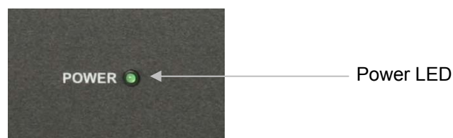
Figure 2: Power light indicates when DV Capture is receiving power.
