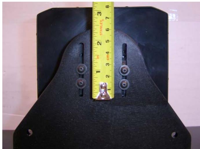
Figure 6: Mounting position for the Canon camcorders - note the Allen screws are in the top two sets of holes of the tilt hub.
